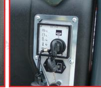
Electric, Key Ignition Start & Led Warning Lamps (Diesel Electric Model)
