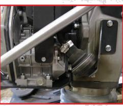
Spark Arrester Option for Diesel Model
