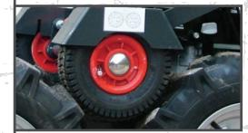
Carrier wheel disengages for easy wheel changing
