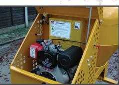
Yanmar L48 'Tier V' Diesel engine'
