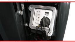
Electric, Key Ignition Start & Led Warning Lamps
