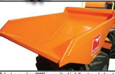
Robust, easy-clean 1000kg capacity skip fully returned edges to prevent dirt ingress
