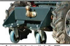
Towing-eye attachment capable of pulling 1000kg ideal for moving trailers, caravans etc.
