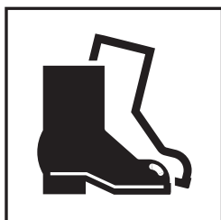
Wear Protective Footwear
