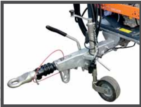
40MM TOWING EYE, BREAK-AWAY CABLE & TELESCOPIC JOCKEY WHEEL / JACK (OPTIONAL 50MM BALL HITCH ALSO AVAILABLE)
