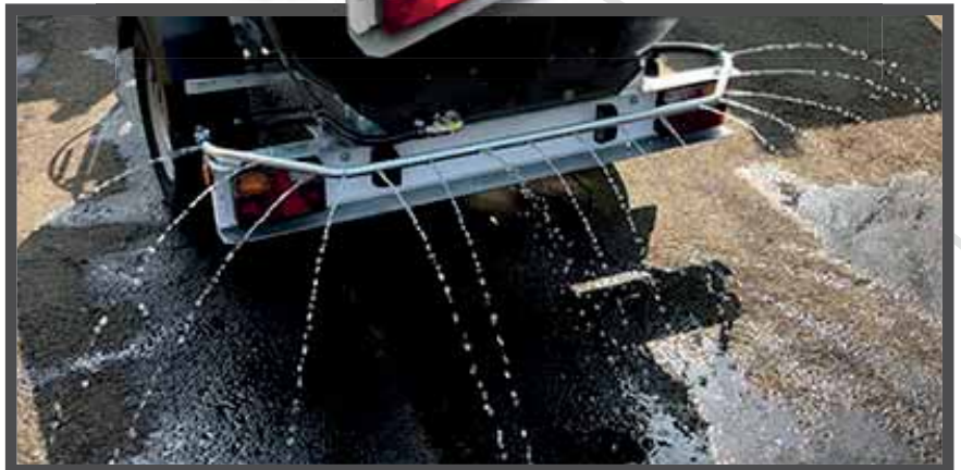
GRAVITY-FED SPRAY BAR OPTION FOR DUST SUPPRESSION
