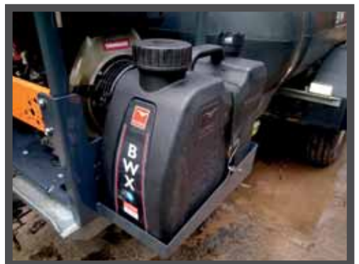
GENEROUS 550MM TANK MOUTH & INTERNAL TANK BAFFLE
