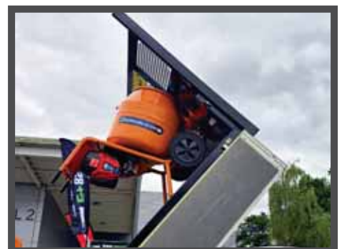
MIXER CAN BE LEFT, SECURELY, ON A TIP-BED DURING TIPPING
