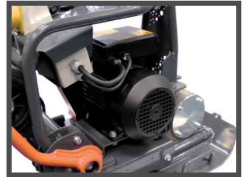
2.2KW ELECTRIC MOTOR & 16KN VIBRATOR
